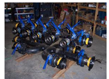
Manifold for a “6 pack” of Upright tanks
